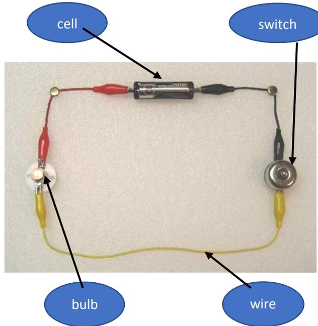
The switch opens and closes the circuit. The bulb lights in this circuit because the switch is on.
